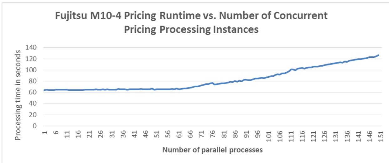
As can be seen in the chart above, the processing performance of the Fujitsu M10 remains very constant from 1 to around 66 simultaneous process instances – barely varying at all. When loaded with higher numbers of processes, the system does slow down, but it’s a very gradual and predictable process, which is what you want from a system. Predictability is the key here, so that the admins know when the processes will complete.
