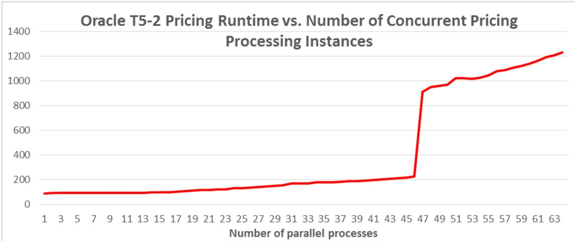
First, note the start point of the line compared to the right axis. While the Fujitsu system started with an average processing time of 65 seconds or so, the Oracle server starts at around 90 seconds – almost 50% slower right off the bat.
